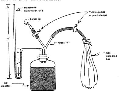
2. The manometer is made from glass tubing and is constructed as is shown in the diagram.
